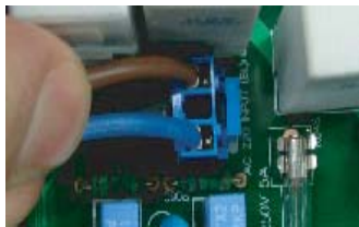
Inverter PCB assembly power connection
