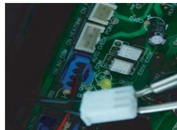
Checking temperature sensor disconnection
