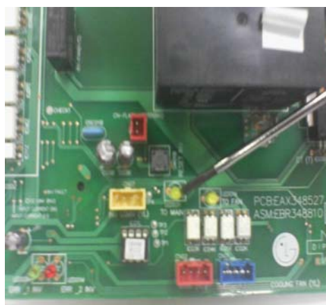
Communication connector & LED in inverter compressor PCB
