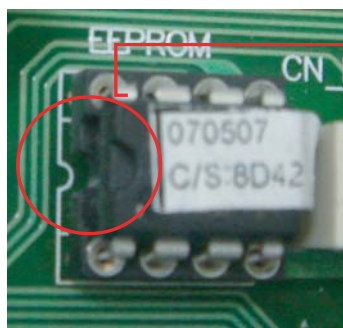
Inverter EEPROM insertion direction
