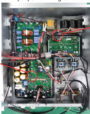
15V input power wiring conditions
