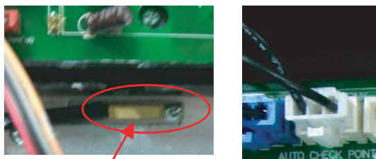
Fan Heatsink assemble position
